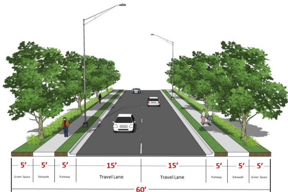
Minor Urban Collector (Type D2) – 2 Lane, 60' ROW, 15' Lanes
